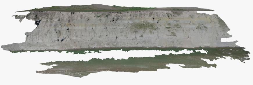
A 3D model based on flight 2. It shows some generalization of the cliff surface thereby indicating a less accurate 3D model. The elevation of the hill was also not taken into consideration in this model.
