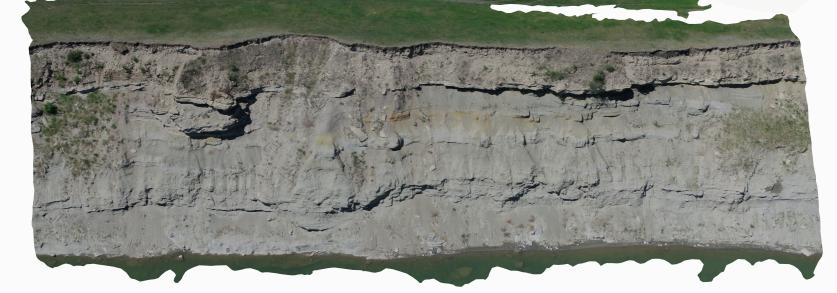
A 3D model based on flight 4. It intentionally disregarded the hill to focus solely on the cliff surface. It therefore produces the most detailed representation of the cliff surface.
