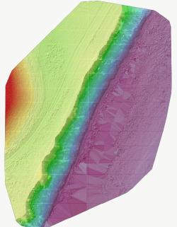
For every X and Y position, the DSM has only one Z value, which The orthomosaic was generated based on orthorectification is the highest altitude of each point in the point cloud. This Z and used the DSM to remove perspective distortions from the value makes the DSM a 2.5D model. It enables the computation images. Distances are preserved within the model thereby making it reliable for measurement. of volumes, the orthomosaic, and the reflectance map.
